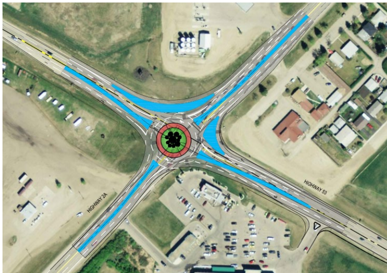
FIGURE 7-5: HIGHWAY 2A & 53 STREET PROPOSED IMPROVEMENTS – ROUNDABOUT
