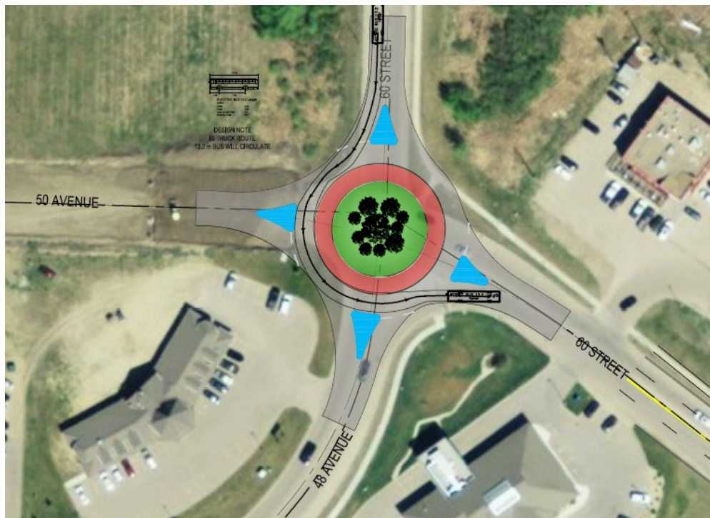
FIGURE 7-6: 60 STREET & 48 AVENUE PROPOSED IMPROVEMENTS – ROUNDABOUT
