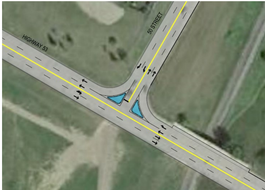
FIGURE 7-2: HIGHWAY 53 & 50 STREET PROPOSED SHORT TERM IMPROVEMENTS
