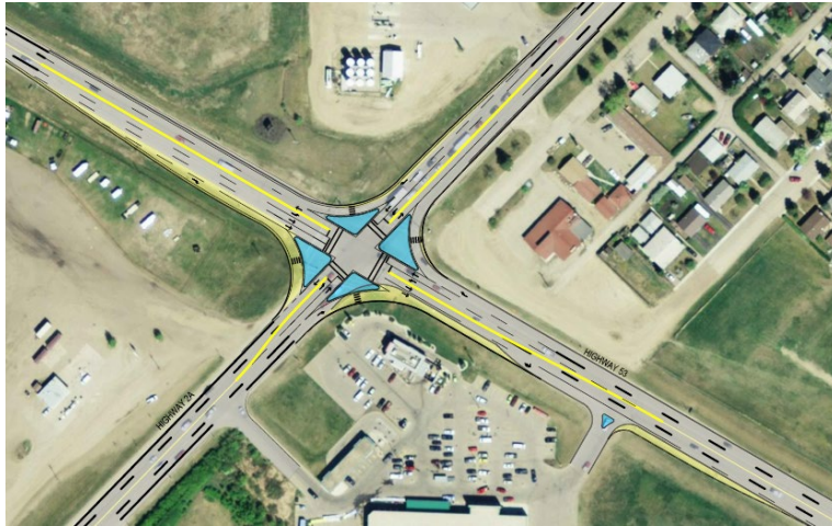
FIGURE 7-4: HIGHWAY 2A & 53 STREET PROPOSED IMPROVEMENTS – CHANNELIZATION
